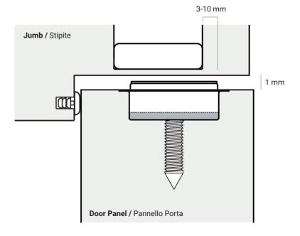
Stoppino Open is a concealed magnetic door-stopper developed for interior doors. It prevents the door from opening too far and damaging nearby wall or furniture or slamming because of the wind
