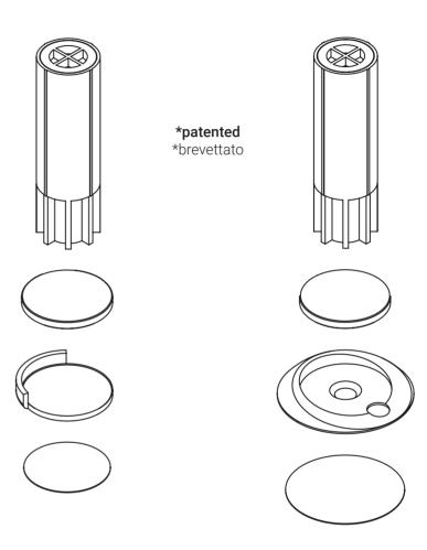
Stoppino Open is a mechanical door-stopper with magnets.
